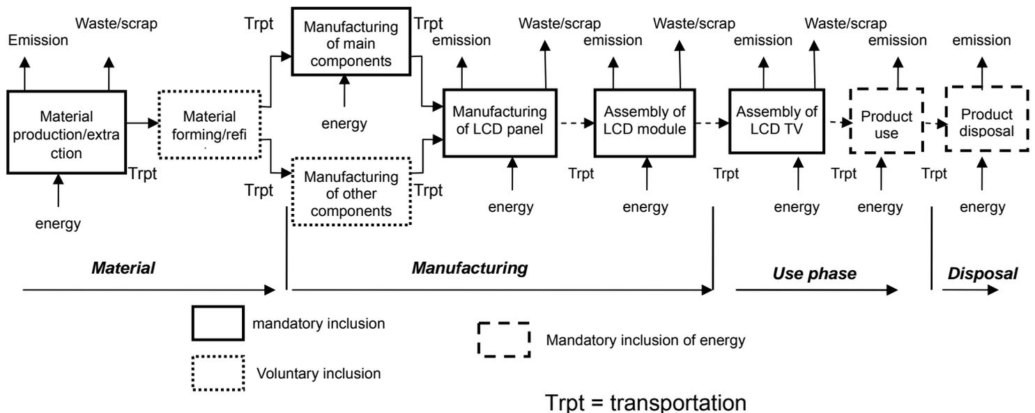
Figure 1 System boundary of the main product system
